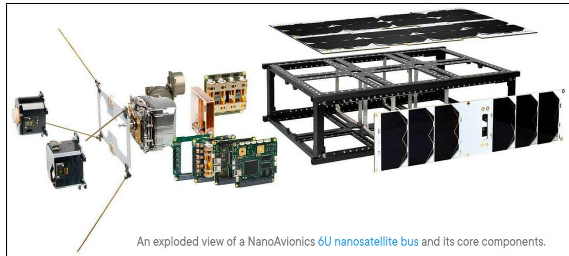
An exploded view of a NanoAvionics 6U nanosatellite bus and its core components.
